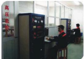
Impulse Current Test 2ms Rectangular Current Withstand Test
